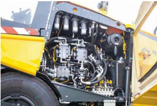
Save up to 17 % fuel – demand-driven hydraulics – with BOMAG ECOMODE.
