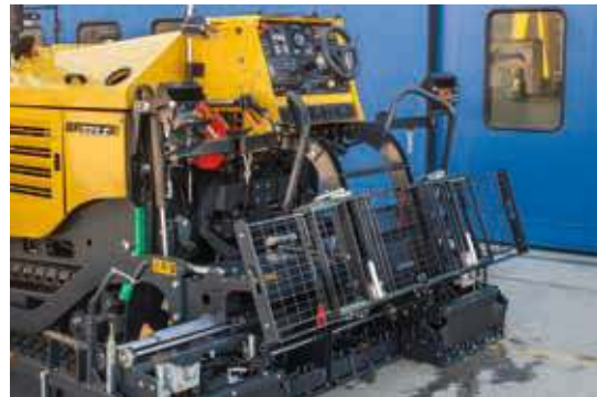
The step plates can be folded up to save space when starting installation near obstacles – extendable to a width of 2.20 m.
