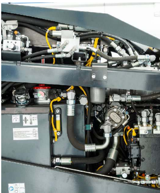
Save up to 20 % fuel – demand-driven hydraulics – with BOMAG ECOMODE.
