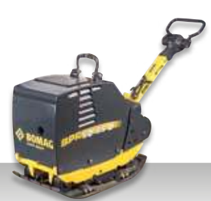
BPR 50/55 D Operating weight: 485 kg Centrifugal force: 50 kN Working width: 550 mm
