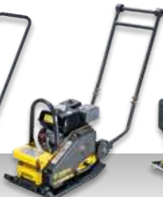
BVP 10/36 Operating weight: 83 kg Centrifugal force: 10 kN Working width: 360 mm
