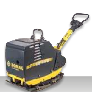
BPR 50/55 D Operating weight: 485 kg Centrifugal force: 50 kN Working width: 550 mm
