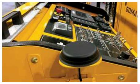
GOMACO Remote Diagnostics transmits through the mobile phone network and picks up the GPS location of the GOMACO machine.
