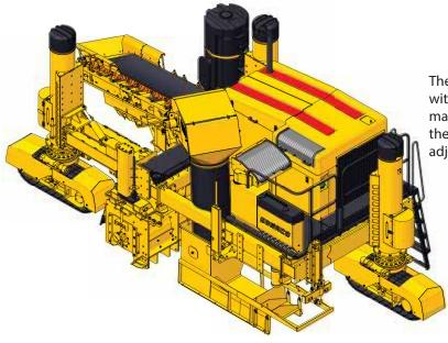
The Commander IIIx features Xtreme Intelligence with the smart hydraulic cylinders on all three of the machine's legs. The smart cylinders allow G+ to know the position of all three tracks, so it can make steering adjustments as needed.
