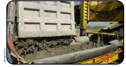
The GOMACO-designed conveyor system on the PS-4000 provides quick, clean and efficient delivery of concrete to the grade. The 5 ft. (1.52 m) wide GOMACO twin conveyor systems are built with the strength and durability to catch the concrete load from end-dump trucks.
