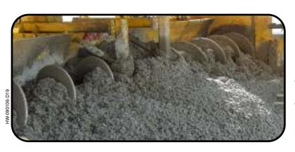
The spreading of either concrete or base material is quick and accurate with the reversible 20 in. (508 mm) diameter hydraulically powered split auger. The hydraulically pressure-compensated sideplates provide edge control and a spreading depth up to 19 in. (483 mm).
