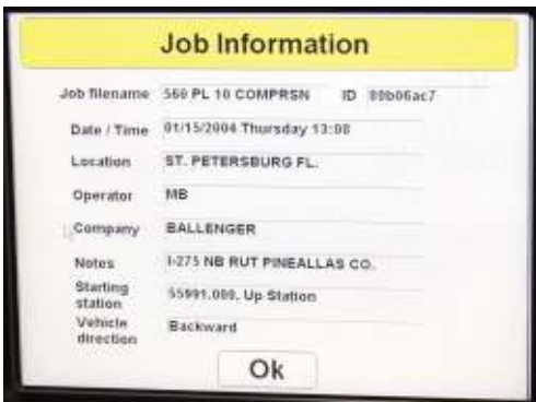
Part of calibrating the system is entering job-site information into the GSI's computer.
