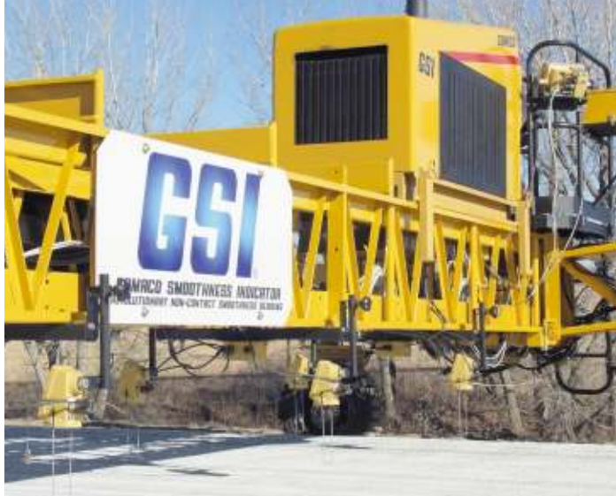
Both sonic and slope sensors mounted to the GSI's frame take readings simultaneously to determine pavement smoothness.
