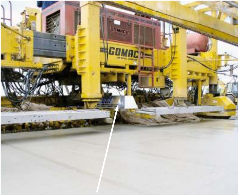
Here, the GSI is mounted to the back of a GP-2600 and in the center of the paver. However, the monitor can be mounted anywhere on the paver for easy viewing.
