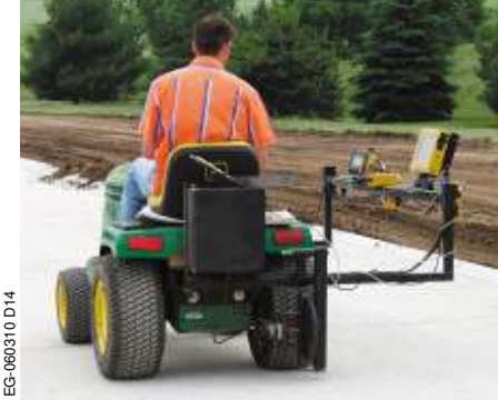
GOMACO's portable GSI package is available for mounting on an ATV or job-site vehicle for a single trace of existing slab or checking stringline. Stringline accuracy can be checked with the GSI equipped with paving sensors.
