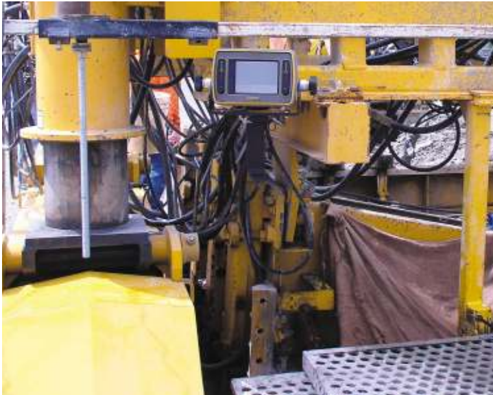
The GSI monitor was positioned on this paver for easy viewing of the smoothness trace from ground level or from the work bridge.
