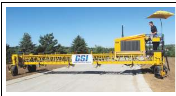
This GSI traces four wheel tracks, providing accurate data for the smoothness readings on this two-lane street.
