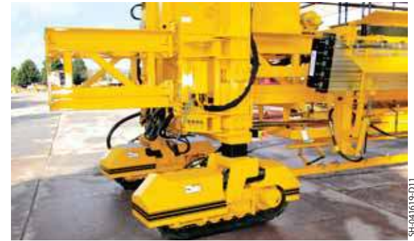
The walking end car allows the T/C-5600 to turn its tracks and walk the end car in or out for additional end sections to be added or removed.
