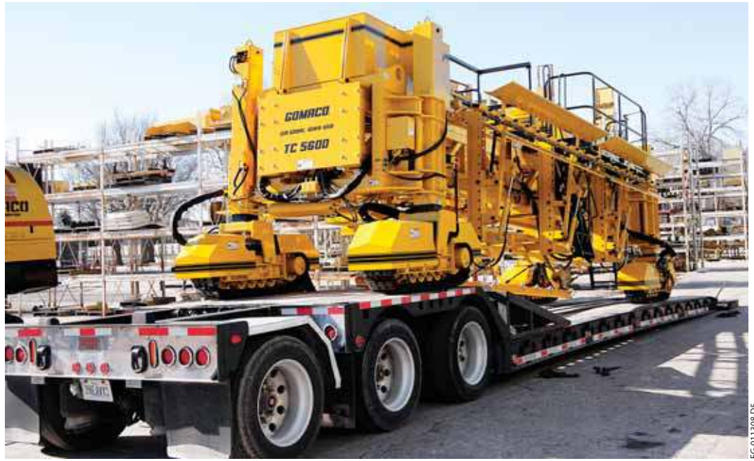
The four-track T/C-5600 texture/cure machine can turn its tracks 90 degrees to drive onto a trailer for transport.
