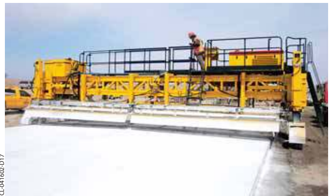
The GOMACO T/C-5600 texture/cure machine has the structural integrity to apply texture and cure up to 56 feet (17.1 m) wide.
