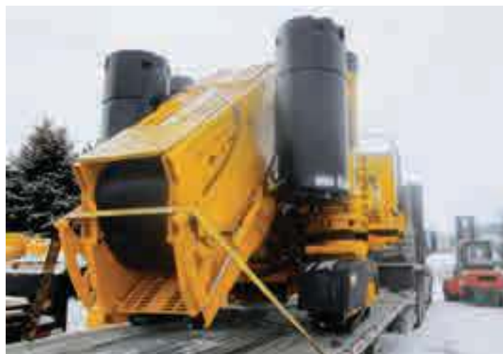
The folding conveyor reduces the transport dimensions on the GOMACO 3300.
